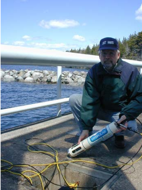
Figure 2. Pumphouse forebay water quality monitoring station. Hydrolab equipment used to collect real-time data.
