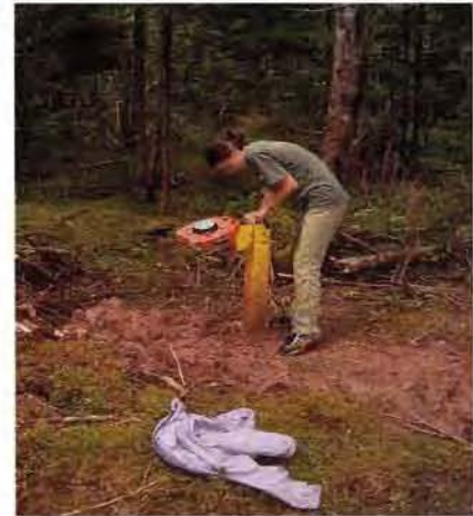
Heather Sutherland, Project Hydrogeologist, sampling water in one of our new observation wells.
