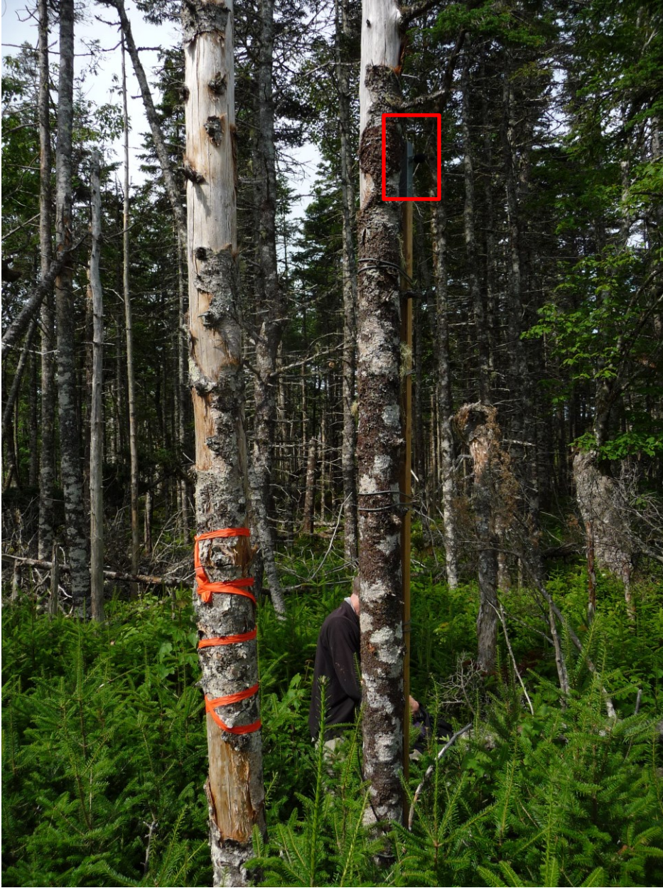
Figure A2. Bat detector (SM2Bat+) placement at site 3 with red rectangle showing the location and orientation of the microphone.
