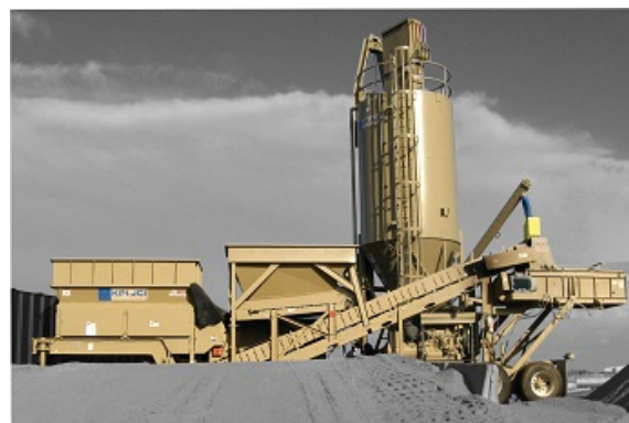
Figure 4 Pictures of Proposed S/S Equipment displaying the Pug Mill System
