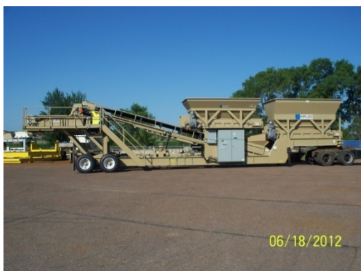
Figure 4 Pictures of Proposed S/S Equipment displaying the Pug Mill System
