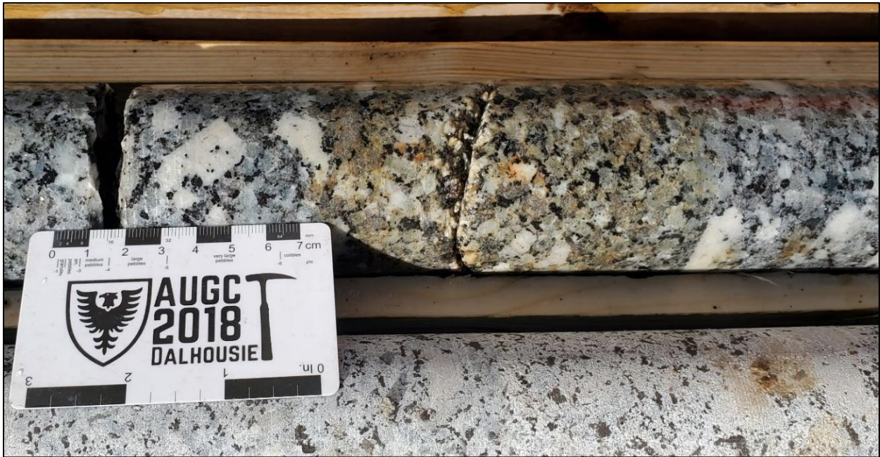
Figure 19: Weak alteration around fracture in the upper portion of borehole BH2 from proposed turbine site T20 - ~4.5 m (14.7 ft) depth.
