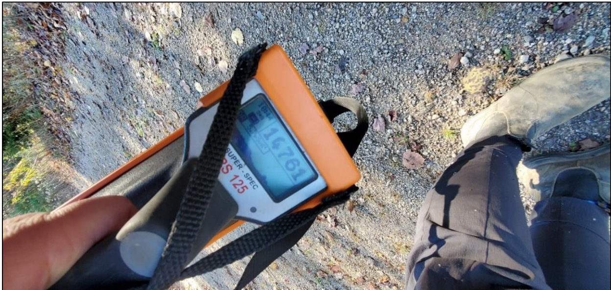
Figure 14: RS-125 Hand-held Gamma Ray Spectrometer reading of 14,761 cps; this measurement was taken along the access road to the Millet Brook Deposit C1 and C2 Zones.
