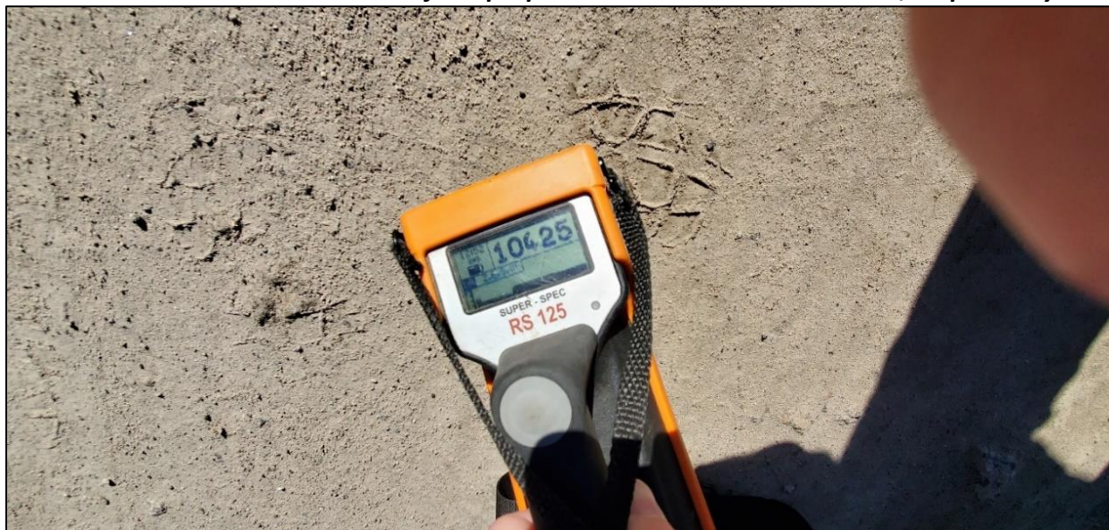
Figure 16: RS-125 Handheld Gamma Ray Spectrometer survey reading of 10,425 cps. This survey measurement was taken within the PDA along the main access road approximately 650 m south-east and 1.5 km south-west of the proposed T28 and T27 turbine sites, respectively.
