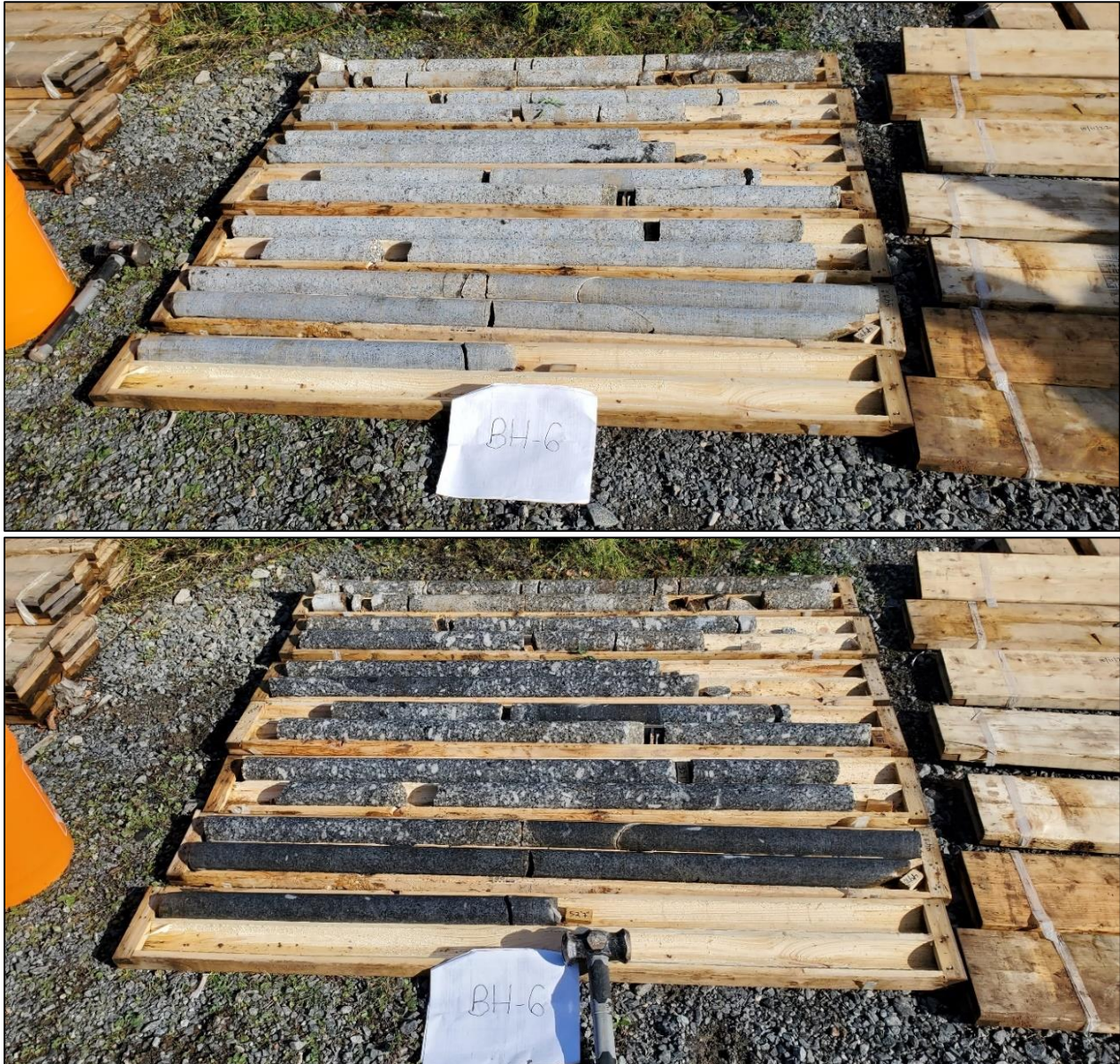
Figure 18: (Top) Photograph of dry borehole BH6 core from proposed turbine site T18, with core boxes organized by depth – top to upper left. (Bottom) Duplicate photograph of wet BH6 core. The contact between the light grey, very coarse-grained biotite granite and dark grey, fine grained biotite granite is clearly seen in the last few meters of BH6.
