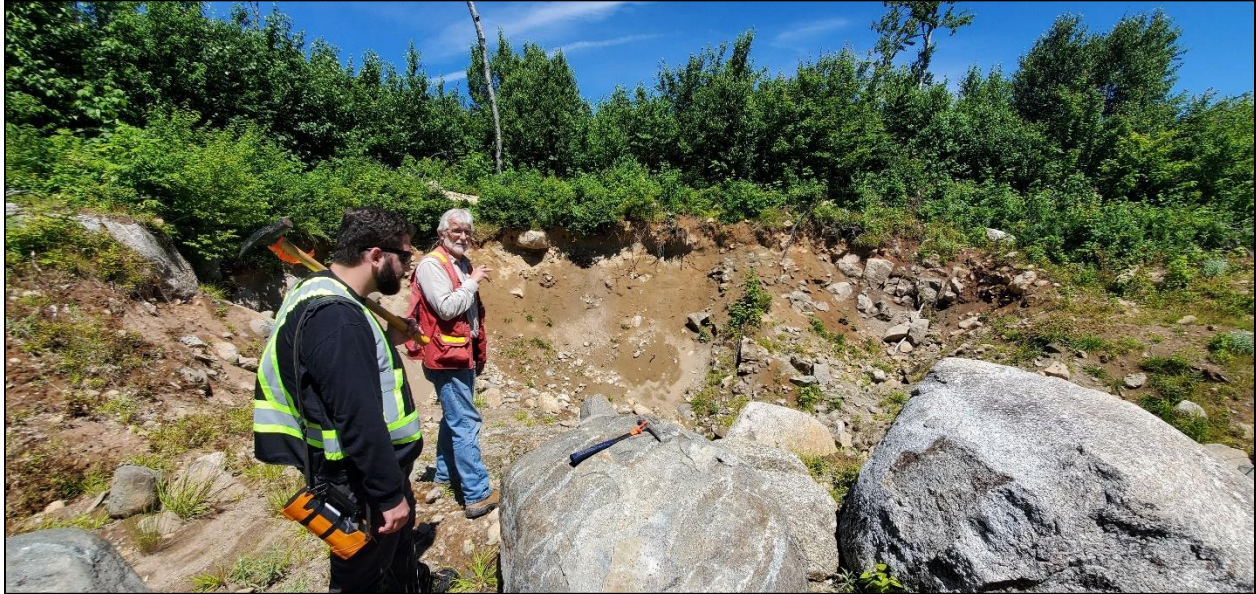
Figure 8: View of the typical surficial and bedrock geology of the PDA – moderately well-rounded large granodiorite boulders with a relatively shallow overburden profile.
