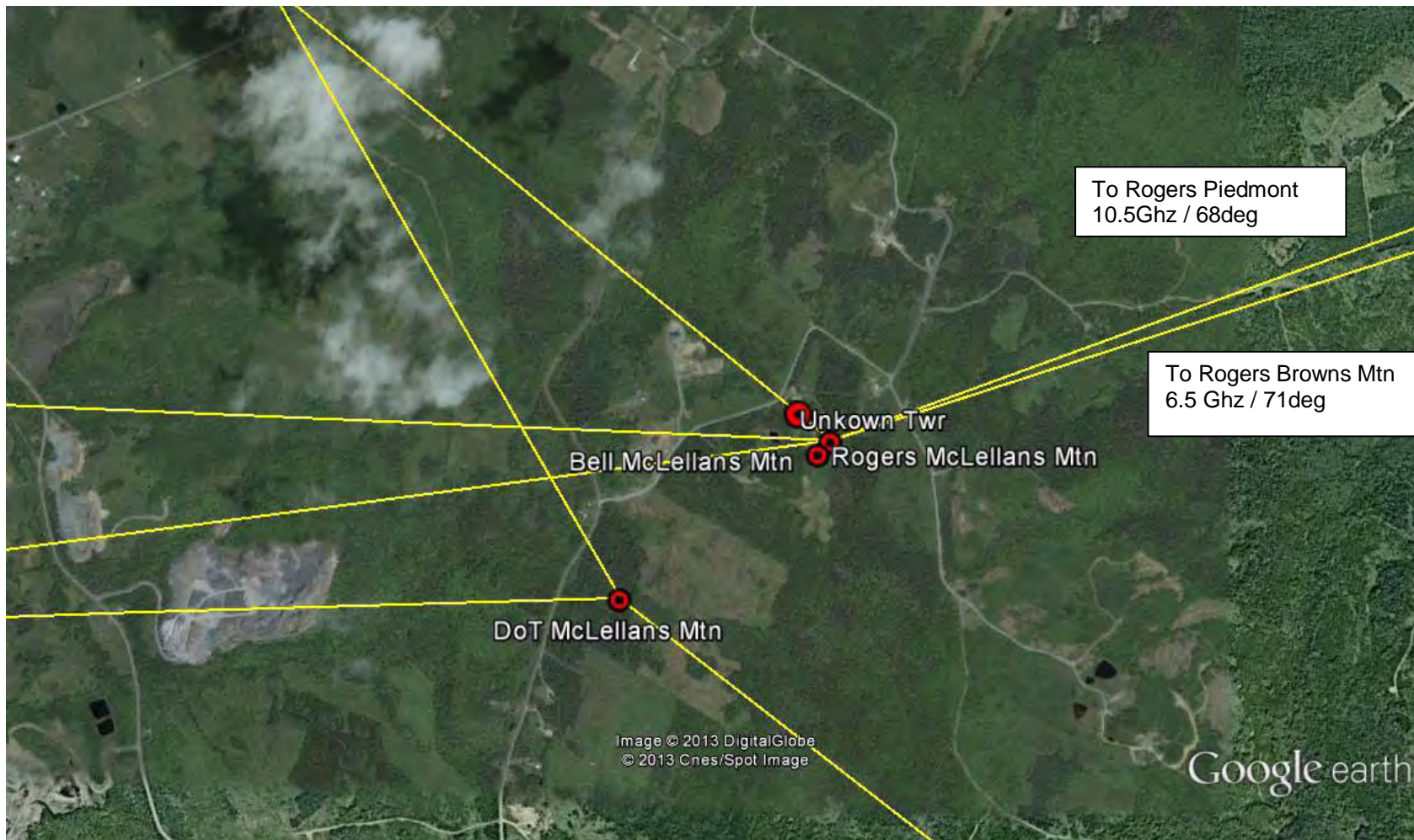
Figure 4 - MacLellans Mountain Radio Sites – Licensed Links To Piedmont Valley (Rogers) and Browns Mtn (Rogers)
