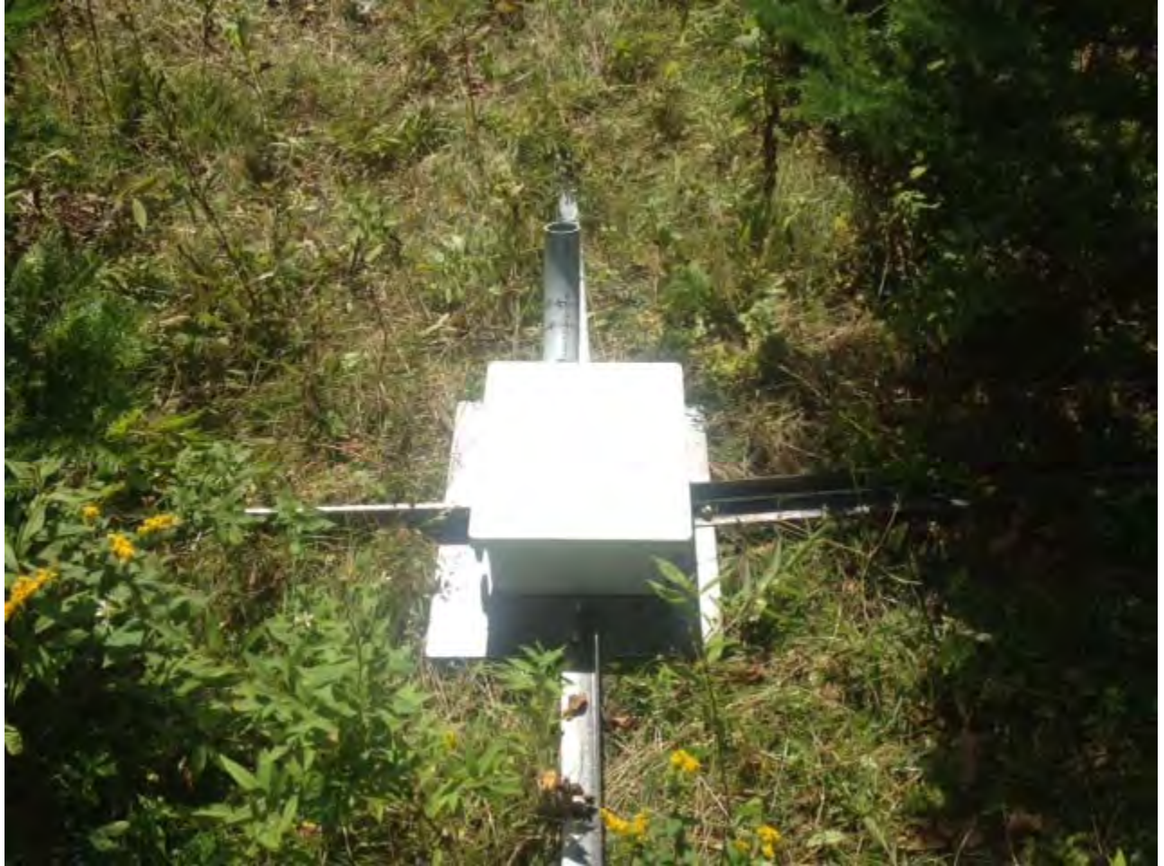
Photo 3.6 Ground Brace which was employed to minimize flipping of Anabat ground units by wildlife.
