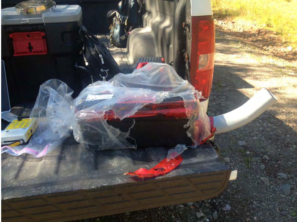
Photo 3.4. Condition on Anabat Ground Unit 2 on Sept 9, showing evidence of damage by wildlife.
