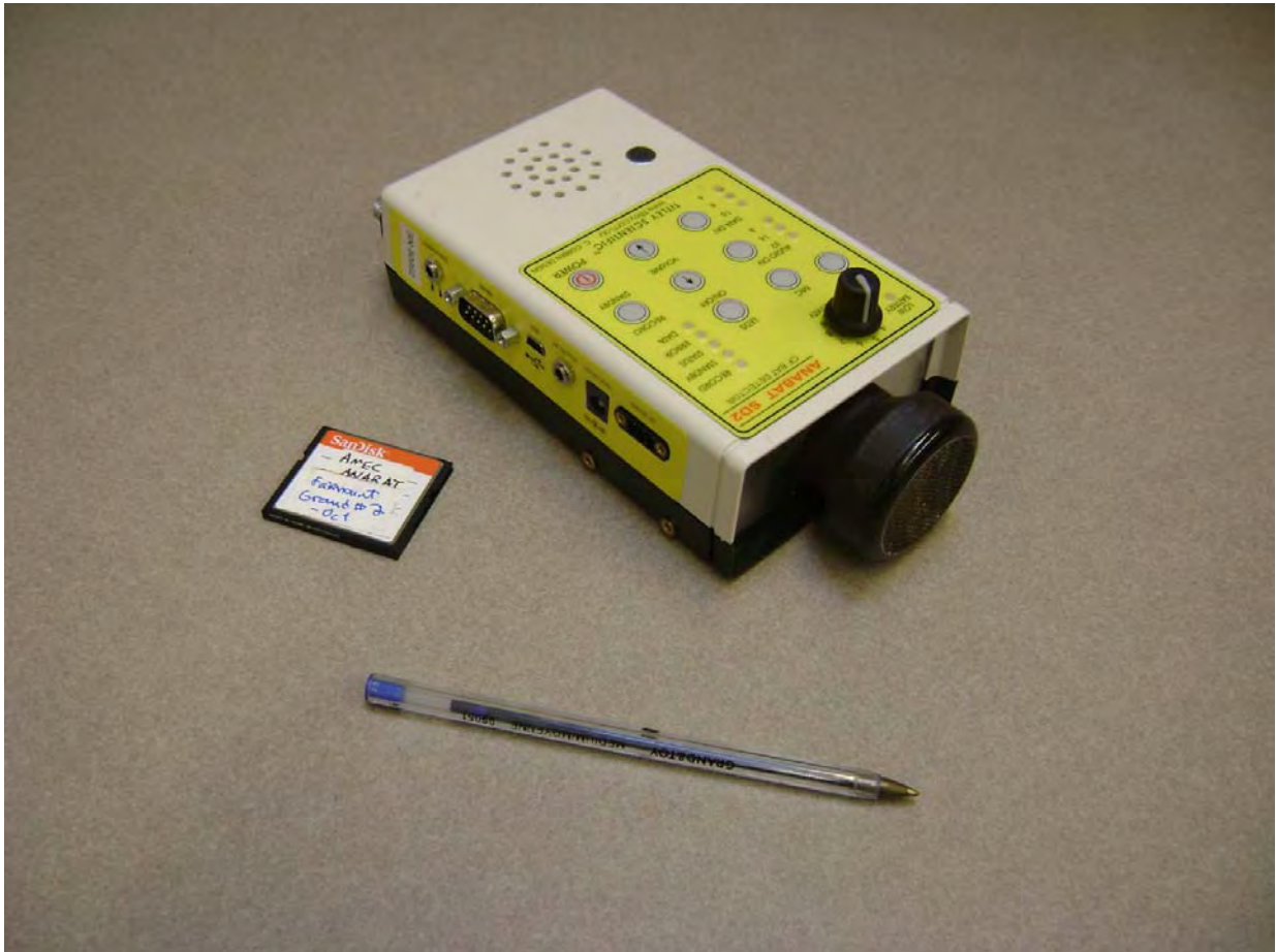
Photo 3.1 An Anabat SD2 acoustic bat detector and compact flash card.
