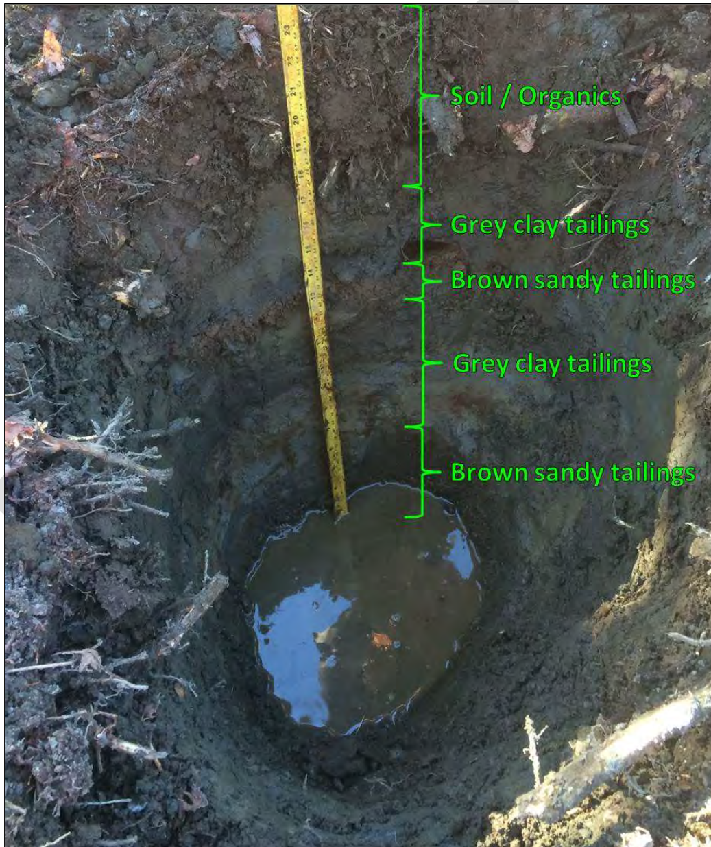
Figure 9: Photo of sample location in the Moose River Gold Mines area showing intercalated clay and sandy tailings.
