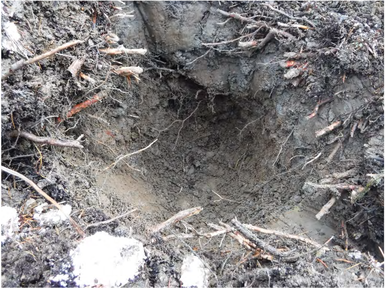
Figure 2 Test Pit GK17-BH16. The following materials were identified: at 0-0.05m below ground surface (BGS) a black organic peat, at 0.05-0.20m BGS a well sorted grey silt (possible tailings) and at 0.20-0.45m BGS a poorly sorted brown silty sand and gravel with cobbles.
