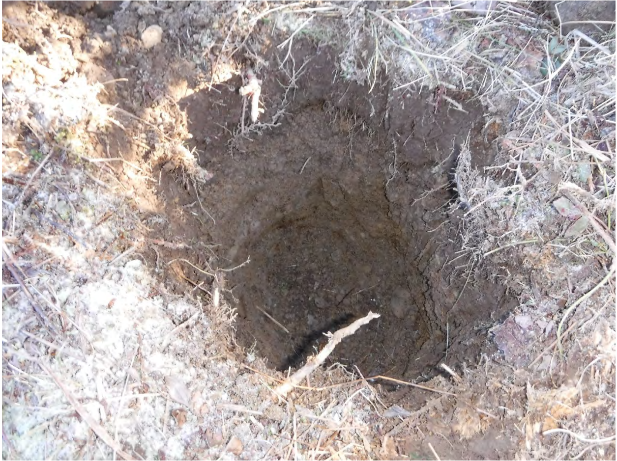
Figure 5 MR17-BH20. Possible tailings were not identified in this location. The following materials were identified: at 0-0.08 BGS grass and rootmat and at 0.08-0.60m BGS a poorly sorted brown silty sand with trace gravel and cobbles.
