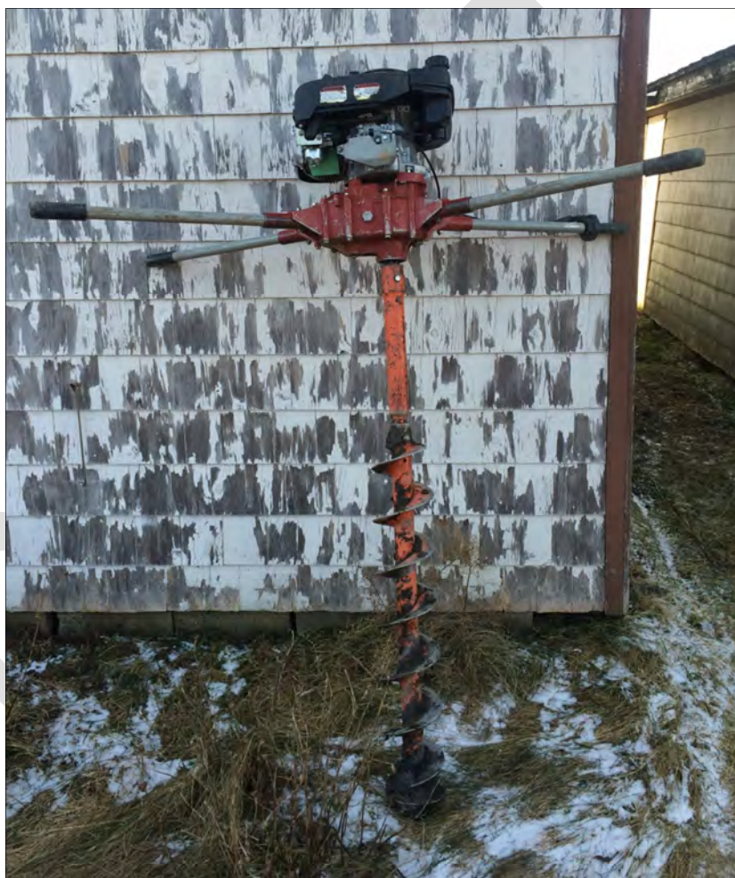
Figure 2: Photograph of gas powered auger used for tailings mapping
