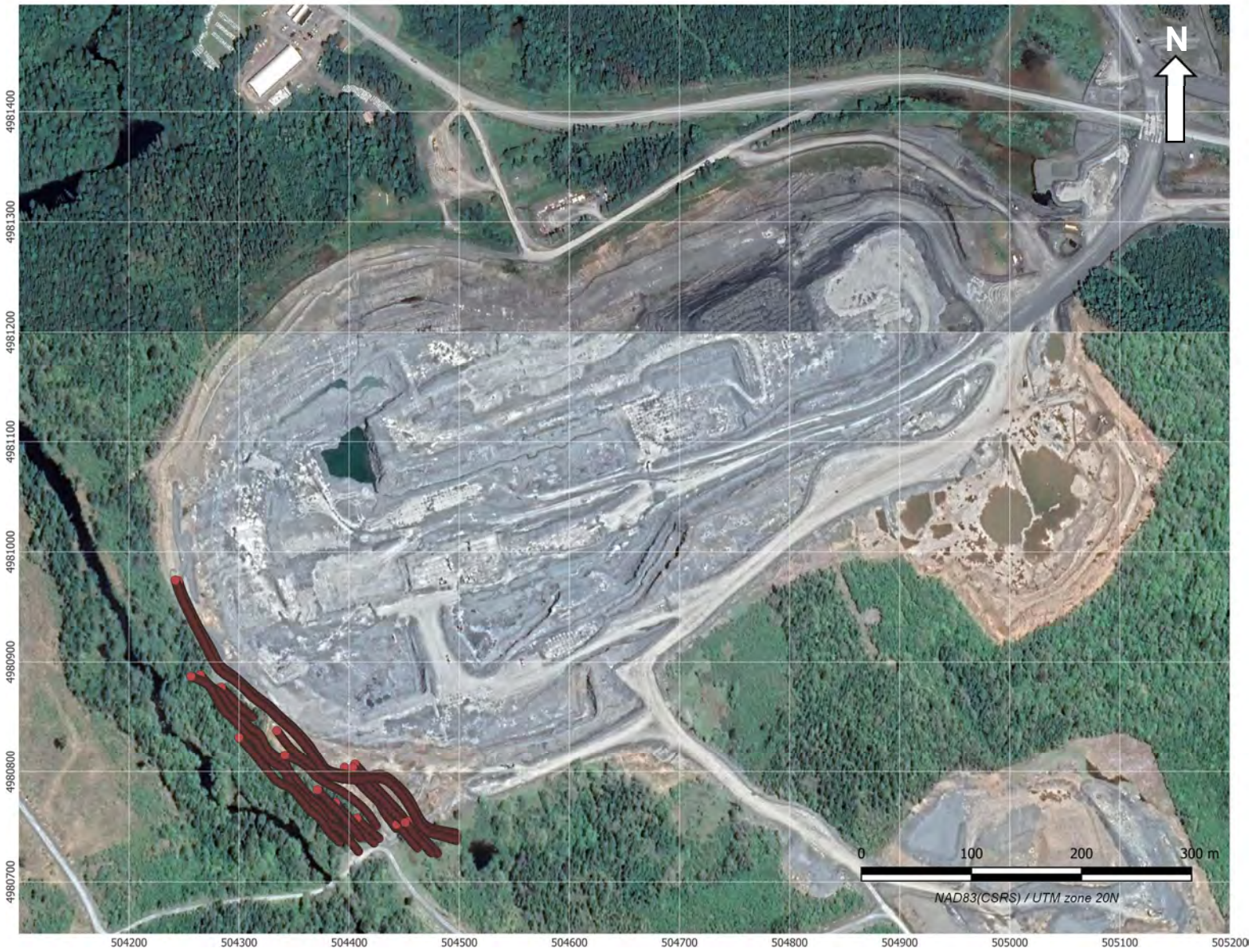
Figure 2. Tracks of the GPR lines (red lines to the southwest) within the greater Touquoy open-pit mine; labelled lines are shown in Figure 3.
