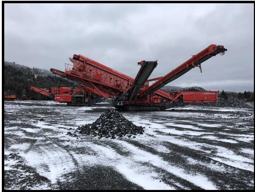
Figure 6: A crusher at the stockpile/crusher area of the Spicer Quarry.
