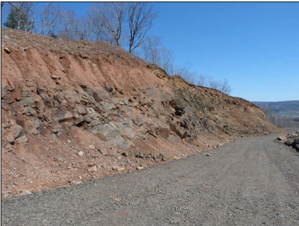
Plate 20: Exposed basaltic bedrock of the North Mountain Formation found along the southeastern extent of the active quarry workings.
