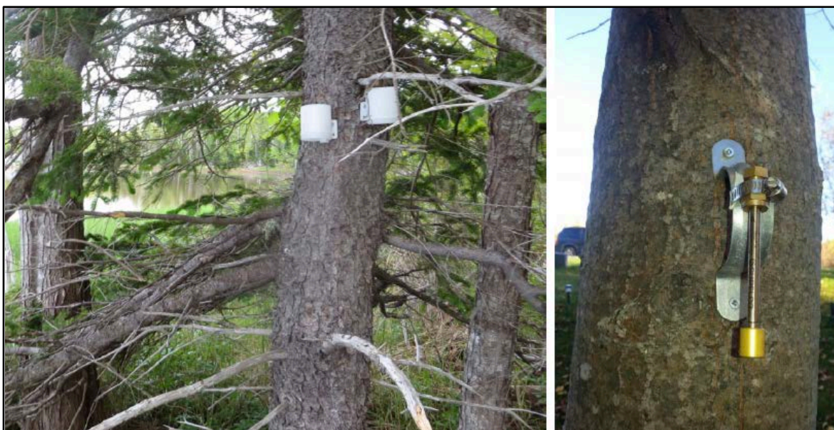
Figure 23. Deployment of passive samplers: Ogawa (left) and thermal desorption tube (right).
