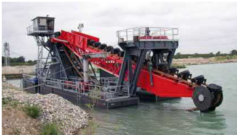
Figure 12. Conventional Excavation Dredging
