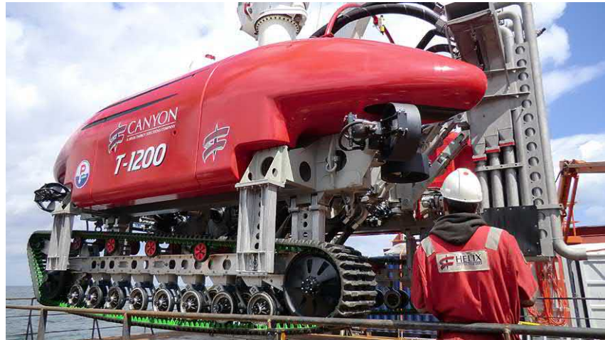
Figure 15. Water jet trenching / burial ROV
