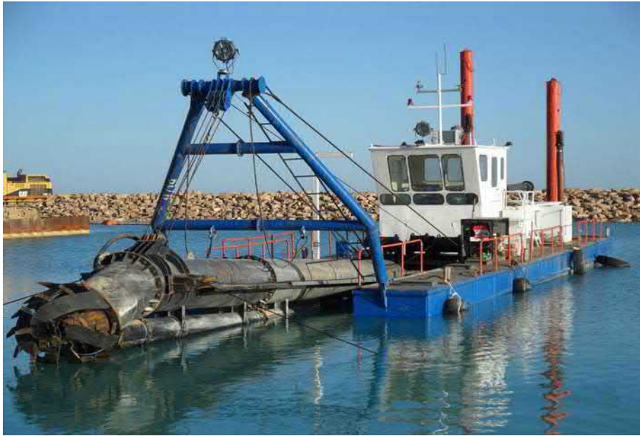
Figure 17. Cutting Suction Dredge
