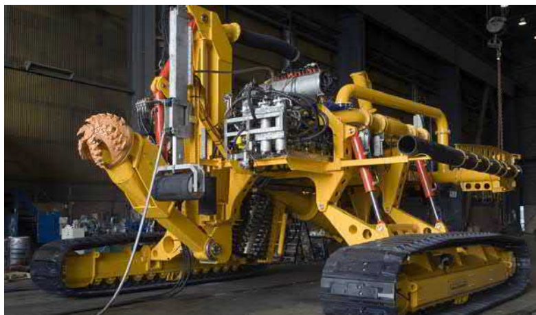
Figure 16. Mechanical Subsea Pipeline Trenching Machine
