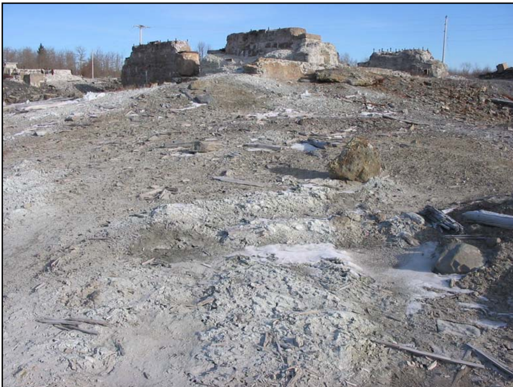
Fig. 4. (a) Cemented remains of sulphide concentrate near the former Dufferin 60-stamp mill in the Salmon River Gold District. (b) Fine-grained, As-rich residue formed through weathering of sulphide concentrate near a stamp mill foundation at Goldenville. The green colour of the residue at both sites is mainly associated with secondary scorodite ( \text{FeAsO}_4 \cdot 2\text{H}_2\text{O} ).
