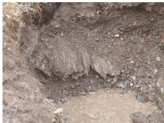
Plate 8-4: Formerly intact bag of oily waste rock encountered in SP10-TP18.
