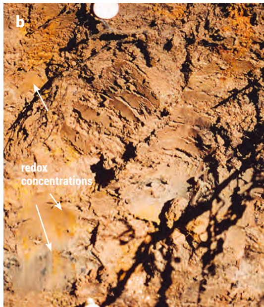
(b) Close-up view of faint to distinct (orange) redox concentrations against a light brown soil matrix.
