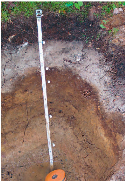
ST3 dominated by sandy loam texture. Note the thick forest floor and well developed (grey) Ae horizon. Redox features are visible in the B and BC horizons in this photo.
