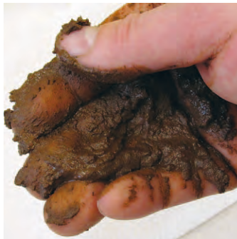
Rubbing sample hard to a thin film between the thumb and fingers to ensure all sand sizes are being assessed – if sample is not rubbed hard, sand content will be underestimated
