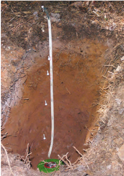
ST5 with a loamy surface layer and clay content increasing with depth (reddish brown colour). Soil type in this stand could shift to ST2-L where loamy conditions extend deeper into the profile (> 50 cm).
