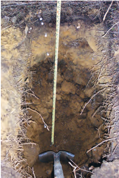
ST1 derived from a sand-capped, gravelly and cobbly glaciofluvial deposit.
