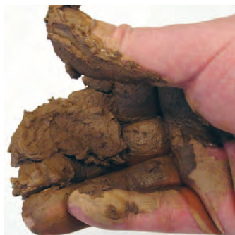
Lifting thumb from fingers to assess relative clay content (stickiness) – if the sample is too dry or too wet, stickiness (clay content) will be underestimated
