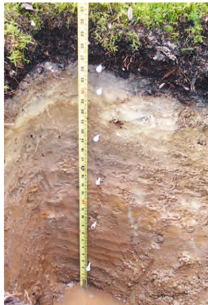
ST3-L derived from a loamy glacial till deposit. L-phase soils often have thinner Ae horizons than most typical soils (as is the case here). Redox features are more noticeable with depth in this photo.
