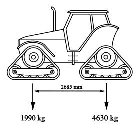
Figure 1 – Design Groomer Axle Load
