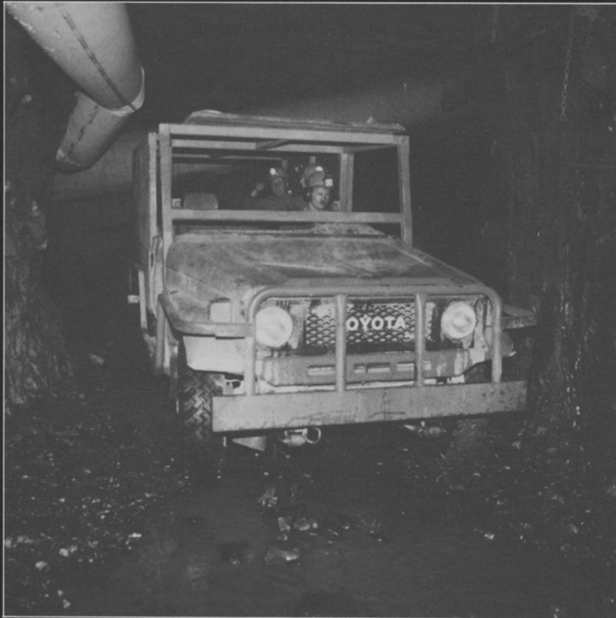
A mining vehicle transporting some of the several dozen miners employed in the underground workings of the Beaver Dam deposit. The ventilation system is seen to the left side of the photo. The mine is operated by Seabright Resources Incorporated.
