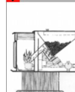
Properly maintained wood pellet stoves burn cleanly and efficiently because the fuel to air mixture can be carefully controlled over a wide range of heat outputs. Pellet stoves need electricity to operate as the fuel is automatically fed into the stove's combustion chamber by a small motorized auger.
