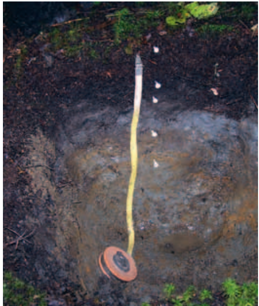
ST4 with a well developed Ae (Aeg) horizon above a depleted B (Bg) horizon with many, prominent redox concentrations.
