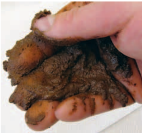
Rubbing sample hard to a thin film between the thumb and fingers to ensure all sand sizes are being assessed — if sample is not rubbed hard, sand content will be underestimated
