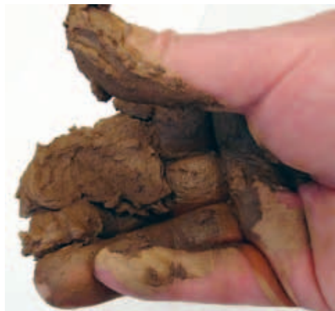
Lifting thumb from fingers to assess relative clay content (stickiness) — if the sample is too dry or too wet, stickiness (clay content) will be underestimated
