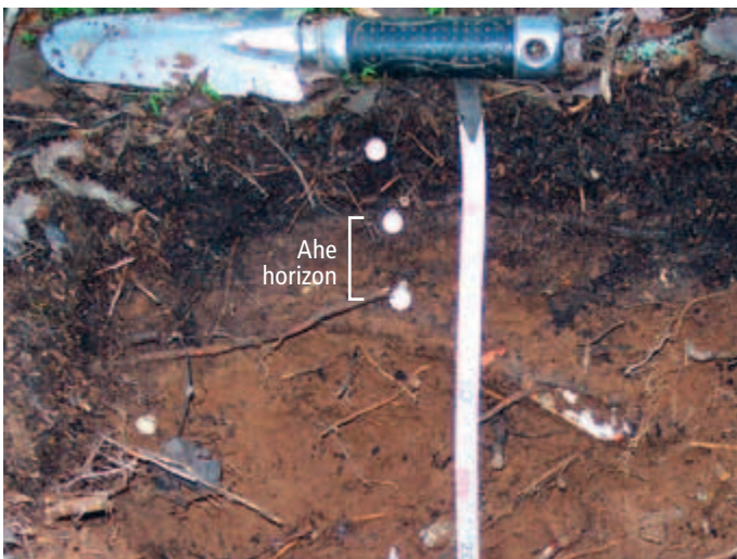
Close up view of a thin, greyish-brown Ahe horizon. Ahe and/or thin Ah horizons are common in ST5 profiles.
