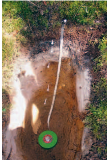
ST1 derived from a sandy glacial till deposit. Note the well developed (almost white) Ae horizon which is common in ST1 soils because of their coarse texture and good internal drainage.
