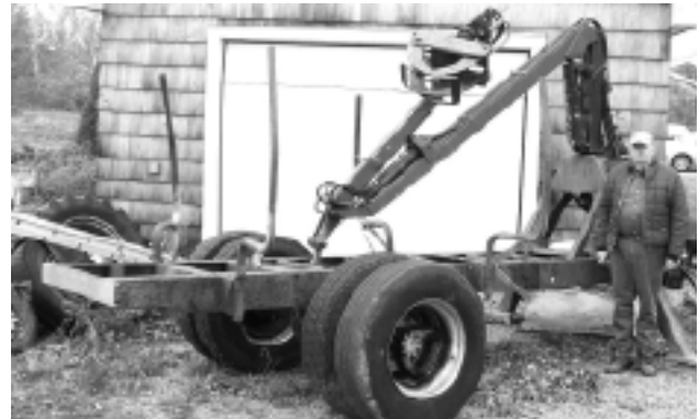
Photo 3.3 Homemade trailer with grapple loader
