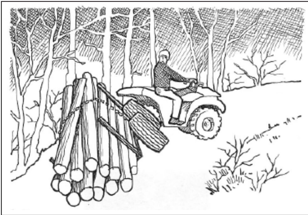
2.2 A rotating hitch saved this driver from overturning too.
