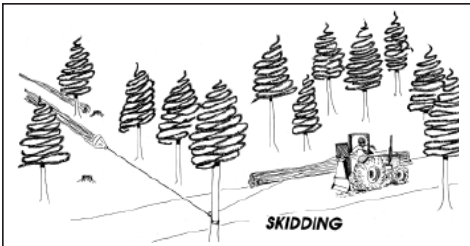
1.2 A tractor has enough power to skid large logs.
