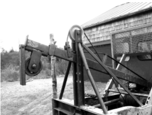
Photo 4.2 The winch cable can lift the boom up and down
