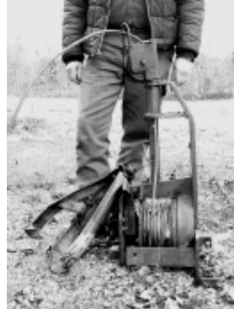
Photo 3.2 Homemade winch (note mast, pulley and grapple)
