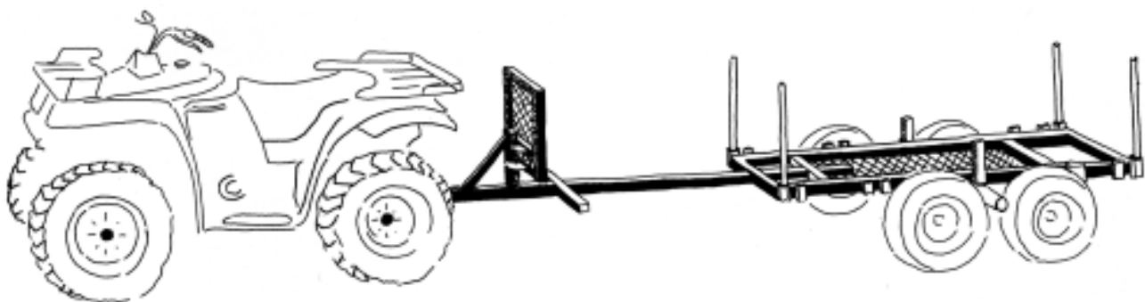
Fig 3.8 ATV trailers should not exceed a maximum load of 600 dg (1,300 lb) and maybe less on smaller ATVs.
